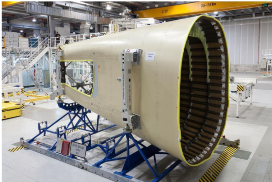
Figure 1.1: A350 section 19 hybrid composite structure (Fualdes, 2016)
