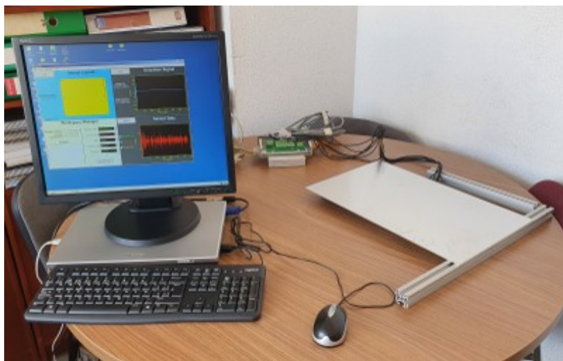
Figure 6: Aluminum plate and DAQ during active interrogation tests.
