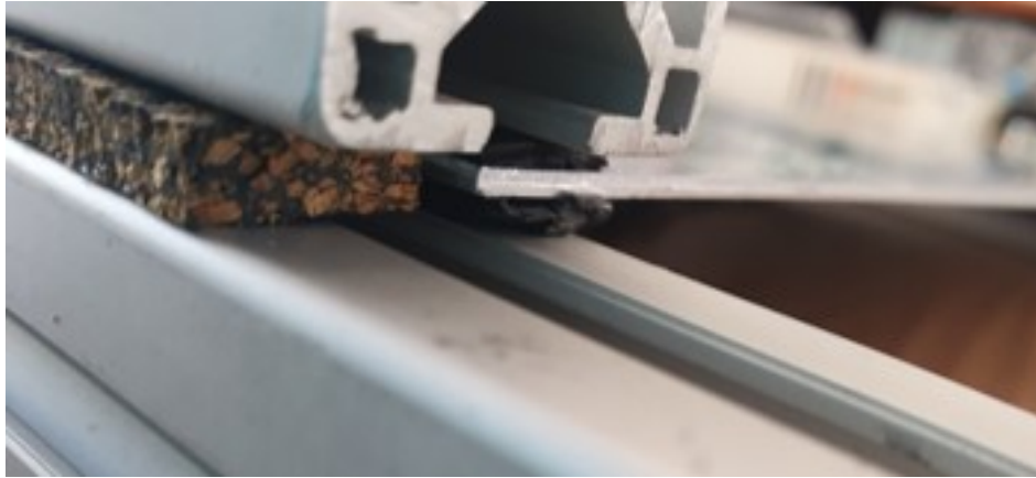
Figure 3.8: Detail of clamped edge and vacuum paste damping setup.
