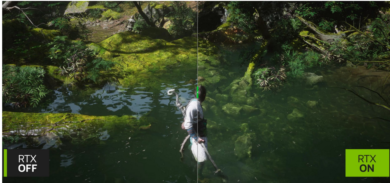
Figure 2.5: Refraction in the water modeled with NVIDIA real-time ray-tracing rendering technology. Left: Without ray-tracing, right: with ray-tracing (Burnes, 2024)
