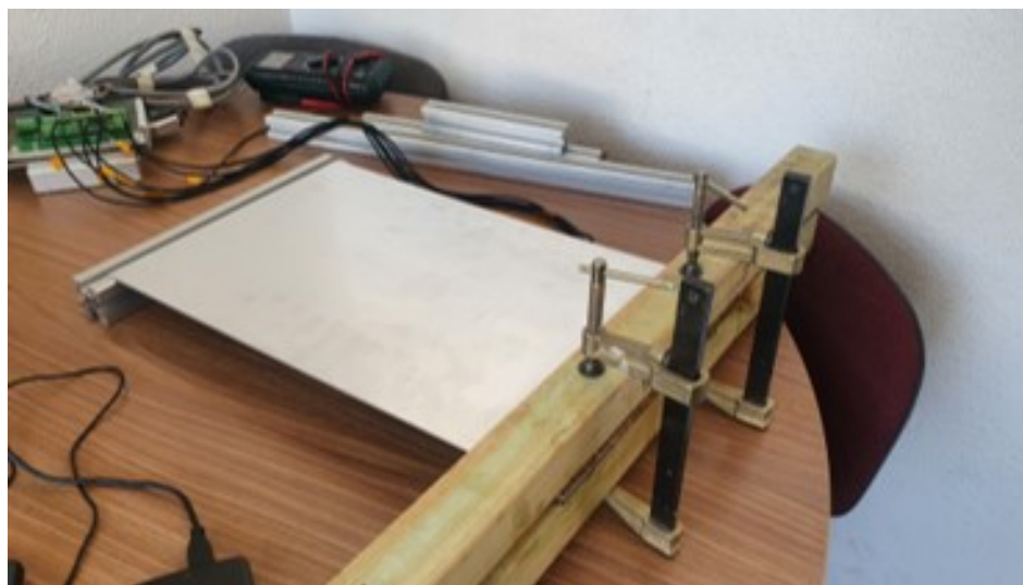
Figure 8: Single edge damped configuration of the aluminum plate for active interrogation tests.
