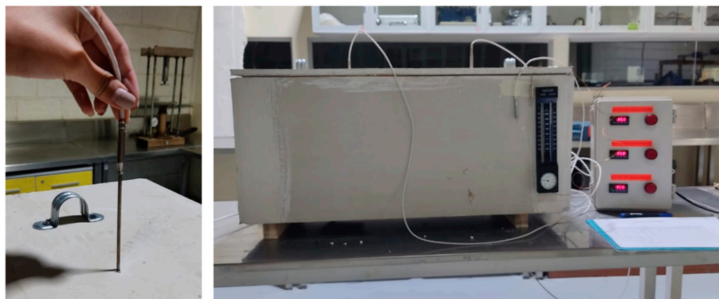
Figure 12. Data collection with thermocouple at intervals of 1, 30, and 60 min.
