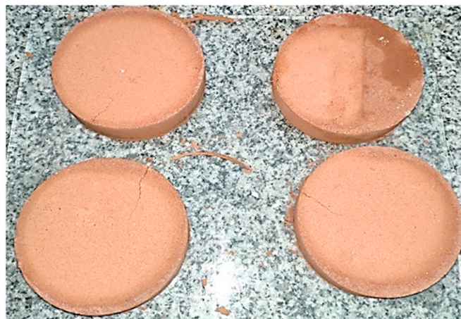
Figure 8. Cracks generated due to excessive curing temperature.
