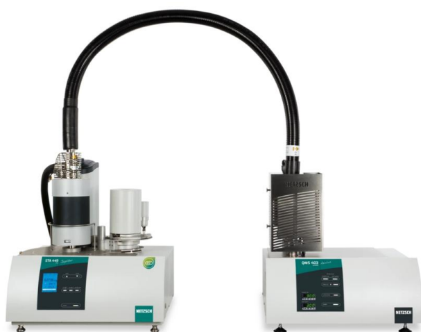
Figure 4.17. NETZSCH QMS403D Aëolos® quadrupole mass spectrometer coupled to the NETZSCH STA 449F5 Jupiter® [160], [161].
