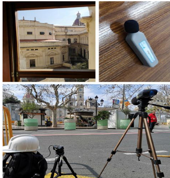
Figure 4.13. Photographs of the locations of the measuring equipment at the Mascletà. Top: Dosimeter 1. Bottom: Sound level meter.
