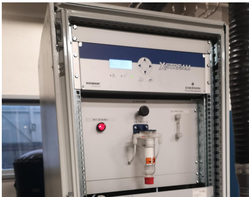
Figure 4.14. Emerson XStreamIR mobile tower gas analyser.
