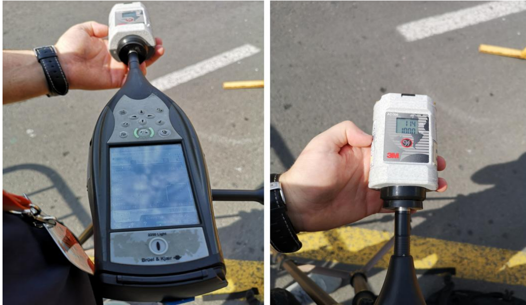
Figure 4.8. Verification of the sound level meter by sound calibrator.
