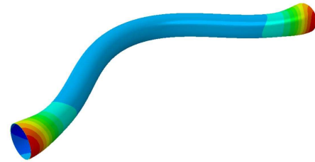
(d) Bulging instability occurring at both ends of the cylinder after bending bifurcation for model associated with figure (b).
