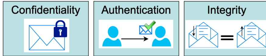
Figure 2.1: Objectives of cryptography: Confidentiality, authenticity and integrity of information.
