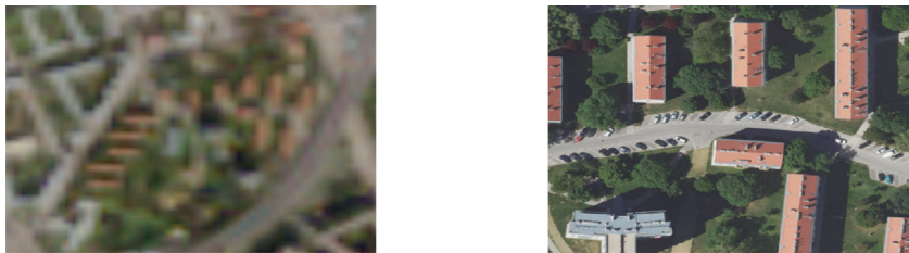
(a) Sentinel 2 10 m resolution image in Vienna (92). (b) 20 cm resolution orthophoto in the same area (6).
