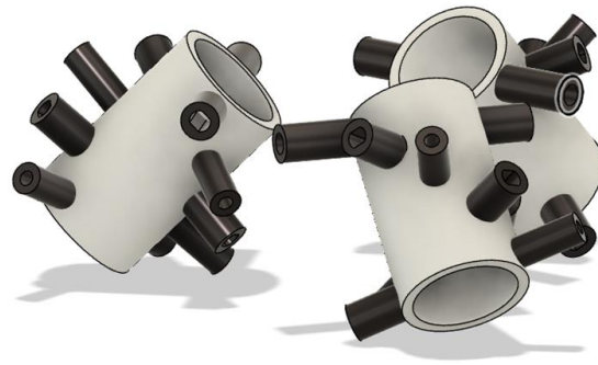
Figure 18. Distribution of sensors for three-dimensional velocity calculation.
