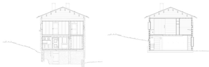
Figure 32. Gugalun House. The plan of the cross sections. The old part (left). The new one (right). Note the direction of the roof rafters parallel to the ridge. Studio Adam Caruso, ETH Zurich (Simon Burri, Grégoire Farquet, Michael Fehlmann, and Lea Hottiger).
