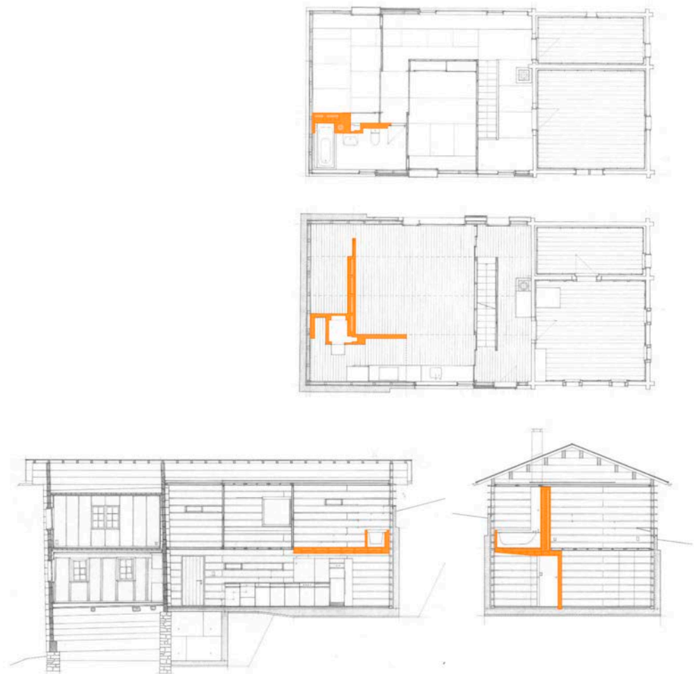
Figure 33. Gugalun House black beast (orange by Silvia Alonso). Note the interior casting of the concrete wall [13].
