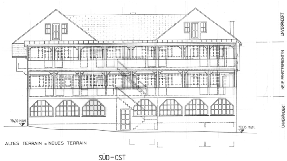
Figure 11. Walenstadtberg Housing. The plan of the southwest façade in their original state (large-dashed line) and their projected state (solid line). Material provided by Gody Kühnis.
