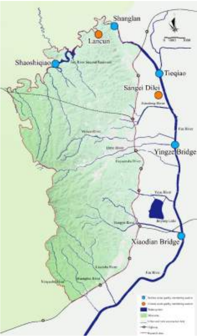
Fig. 74 Surface water monitoring point setting Source: Author’s own work
