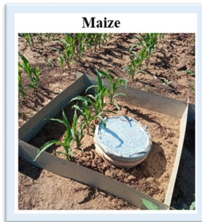
Figure 3.16. Location of the manual static chambers used for gas sampling after maize fertilization and until maize harvest (P2) of Experiment 3.
