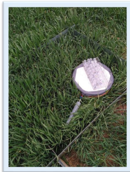
Figure 3.13. Location of the manual static chambers used for gas sampling in the barley crop of Experiment 1.
