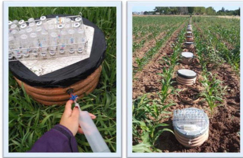
Figure 3.14. Location of the manual static chambers used for gas sampling in the barley cover crop (left) and in the maize cash crop (right) in Experiment 2.
