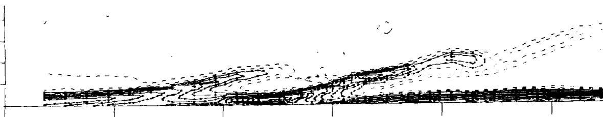
FIG. 5 Vorticity ( \omega_z ) map of an x - y section of ejection structures in the KMM channel. Dotted lines: \omega_z = -1.1 and 0; dashed: 1.1 and 2.2; solid: 3.2 to 17.3. Average vorticity at wall: \bar{\omega}_z = 7.7 . Each horizontal tick mark represents one half channel width ( x^+ = 180 ), each vertical one, y^+ = 17.5 . (From Jiménez et al. , 1988).
