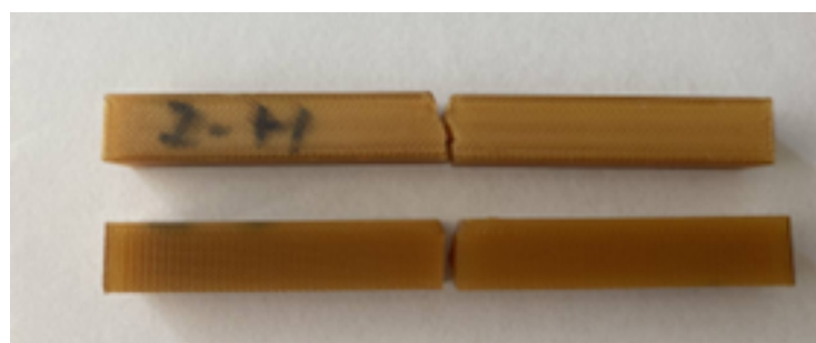
Figure 19. ULTEM™ 1010 Charpy impact samples, notch sideways (top) and notch upright (bottom).
