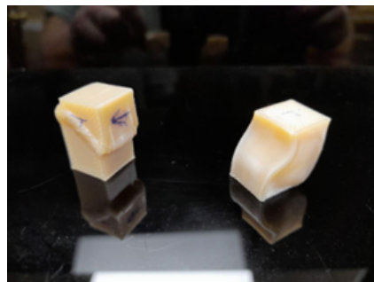
Figure 15. ULTEM™ 9085 compression samples. Flat sample on the left and upright sample on the right.
