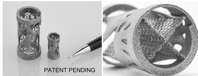
Figure 21. C-flex pivot made through additive manufacturing for PULSAR (figure taken from Kiener et al. [66]).
