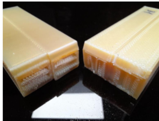
Figure 18. ULTEM™ 9085 Charpy impact samples, notch sideways (left) and notch upright (right).
