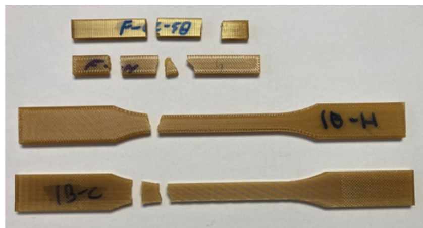
Figure 20. Broken ULTEM™ 1010 samples.
