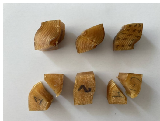
Figure 17. ULTEM™ 1010 compression samples. Upright samples on top, flat on bottom.
