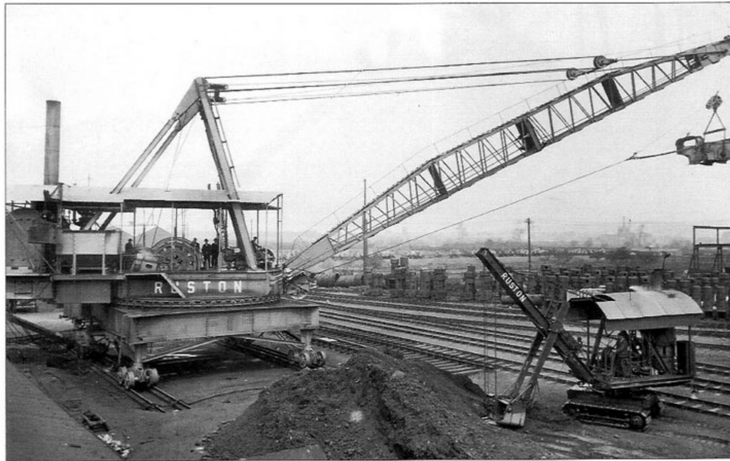
Above: Ruston No.300 Steam Dragline in the Works yard in 1924 dwarfs the Ruston No.6 Steam Crane Navy.
