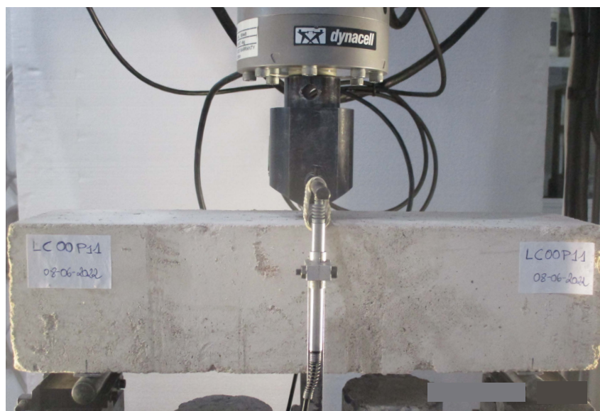
Figure 2. Configuration for a three-point bending test setup.
