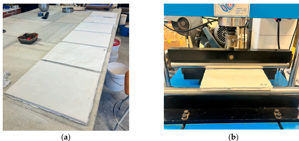
Figure 4. Samples elaborated for flexural strength test. (a) Dried samples; (b) test performed.
