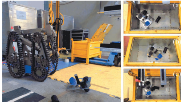
Figure 5.12: Mock-up trials of recovery scenarios at CERN. The robotic system used is not specific for failure managing, but the procedures being tested have been developed specifically for these situations. (Ferrari et al., 2022)
