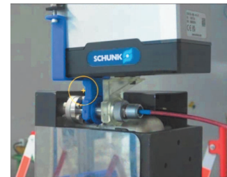
(c) Connector plugged.
