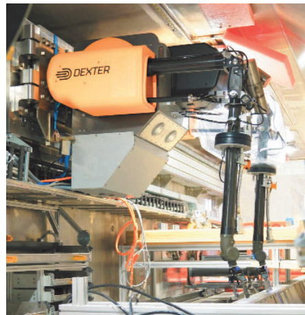
(b) Dexter rad-hard robotic system developed by Veolia. (Veolia, n.d.)
