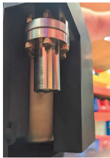
(a) Female part of the electrical connector.
