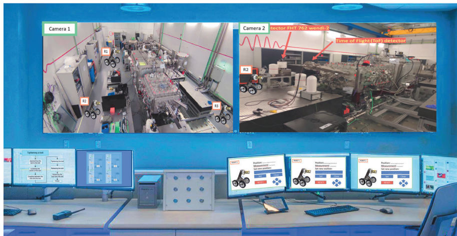
Figure 2.4: Control room for a maintenance procedure using supervisory control and a high automation level. The screens show the information operators need to supervise the ongoing activities.
