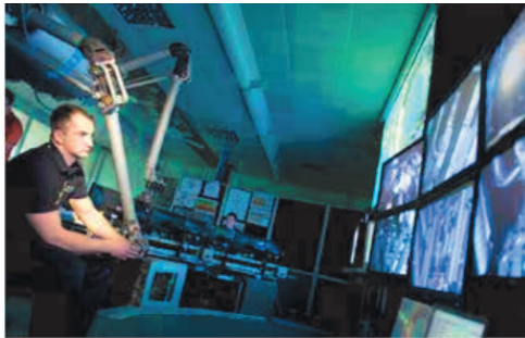
(a) Operator at JET controlling manually the robotic system to perform maintenance procedures.
