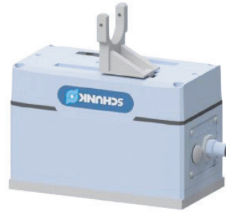
(b) View of the finger for grabbing the male part of the connector fixed to the gripper. It moves along the path when the gripper is open or closed.
