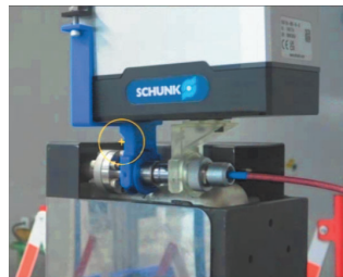
(b) Beginning of the insertion of the male part in the female one.
