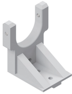
(a) View of the designed finger for grabbing the male part of the connector. It includes spring plungers in its top ends to enable the passive grasping of the connector.
