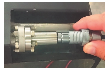
(c) Electrical connector unplugged hands-on.
