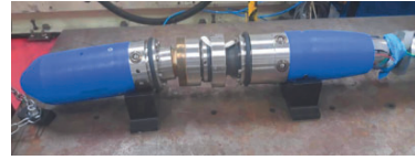
(b) Laser in-bore welding tool developed by UKAEA for DEMO maintenance. (Kirk et al., 2018)
