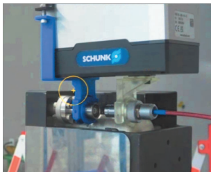
(a) Approach of the male part of the connector to the female one.
