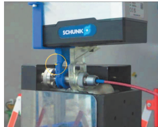
(b) The gripper attaches the connector thanks to the vertical approaching movement of the robotic arm.
