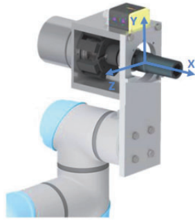
(a) The bolting axis is parallel to the rotation axis of the last joint of the robotic arm.
