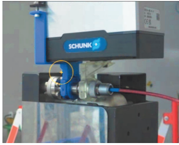
(a) Extraction of the male part of the connector.
