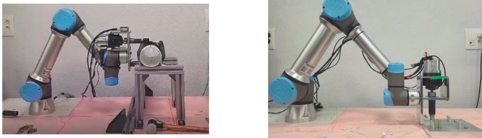
(a) Test bench of the second configuration of the bolting tool. (b) Test bench of the first configuration of the bolting tool.
