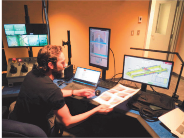
Figure 3.1: In ARIEL the operator can control the hall crane thanks to the visual feedback and the readings of the mechanical encoders in the bridge, trolley and hoists. (Minor et al., 2021)
