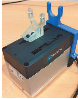
(b) 3D printed designed fingers installed on Schunk EGK50 gripper.
