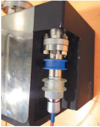
(a) Connector plugged including the 3D printed designed collars.
