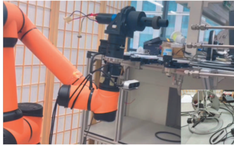
Figure 5.2: Robotic bolt loosening tool. This is an example of a tool designed only to perform unscrewing operations. (Lai et al., 2023)
