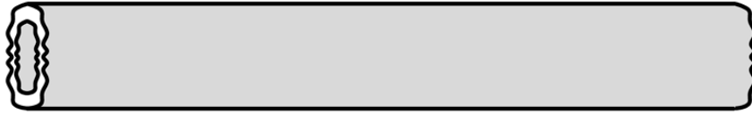
Figure 4.3: Prismatic bifurcation of an initially circular cylinder.
