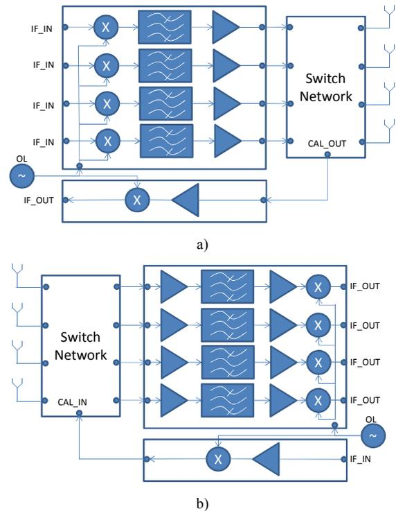
Fig. 4. RF chains with the calibration module at a) transmitter and b) receiver.
