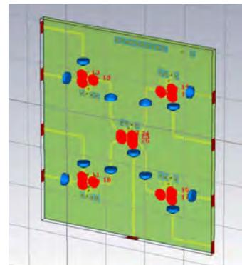
Fig. 1 Switching network of the calibration module.
