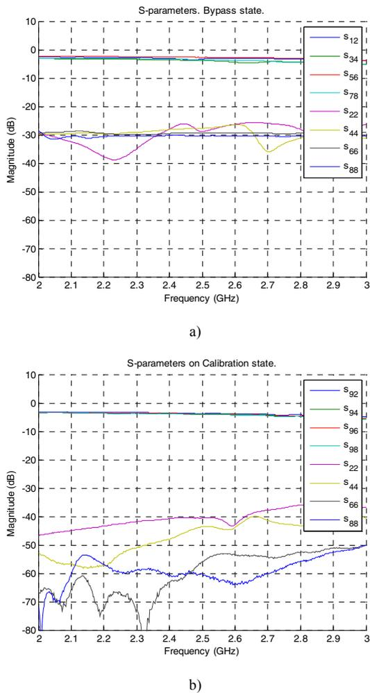
Fig. 2. Measured s-parameters of switching network in a) bypass and b) calibration state.
