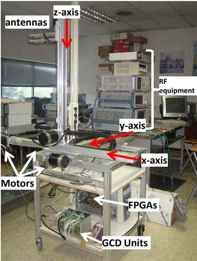
Fig. 5. 3D antenna positioning system for spatial exploring.
