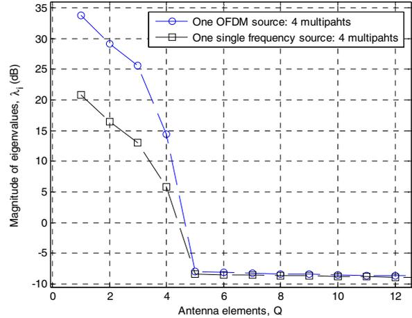
Fig. 8. Eigenvalues calculation using OFDM and single-frequency transmitted signals.
