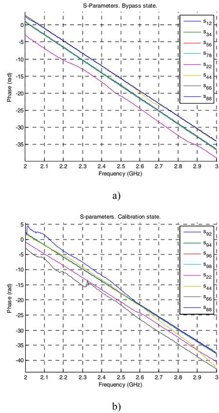
Fig. 3. Measured phase response of switching network in a) bypass and b) calibration state.
