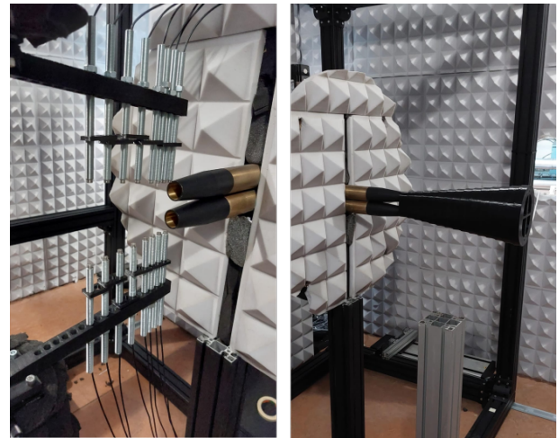
Figure 2. T200 experimental setup: (left) twin-jet system with linear microphone arrays installed; (right) twin-jet system with the 3D-printed part used for microphone positioning.
