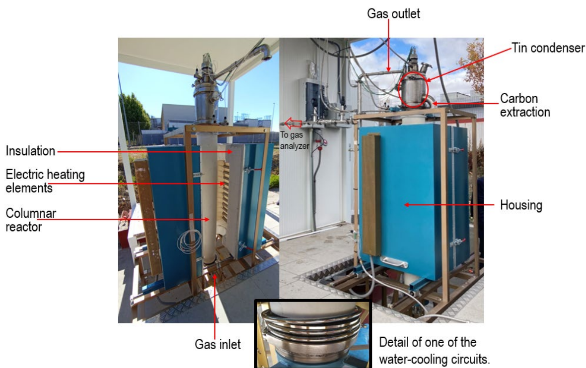
Figure 1. General views of the reactor facility with the heating system open and closed.
