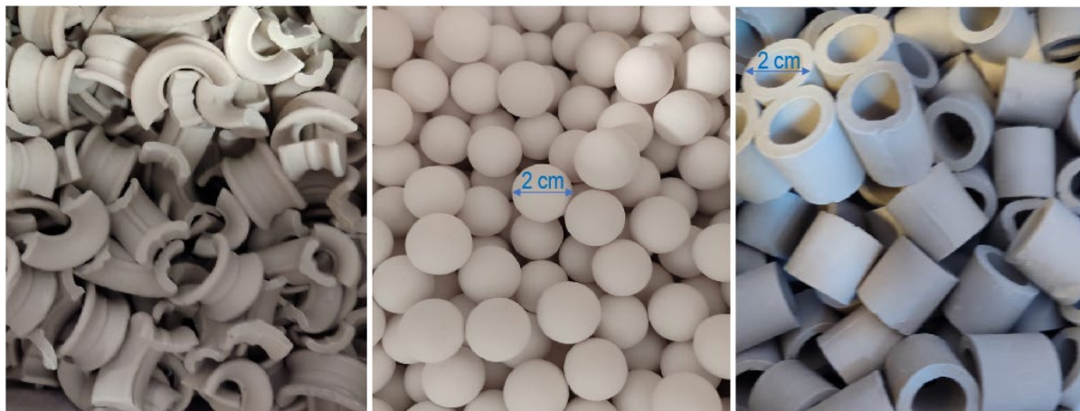
Figure 2. Different shape filler to increase residence time within the liquid metal column.
