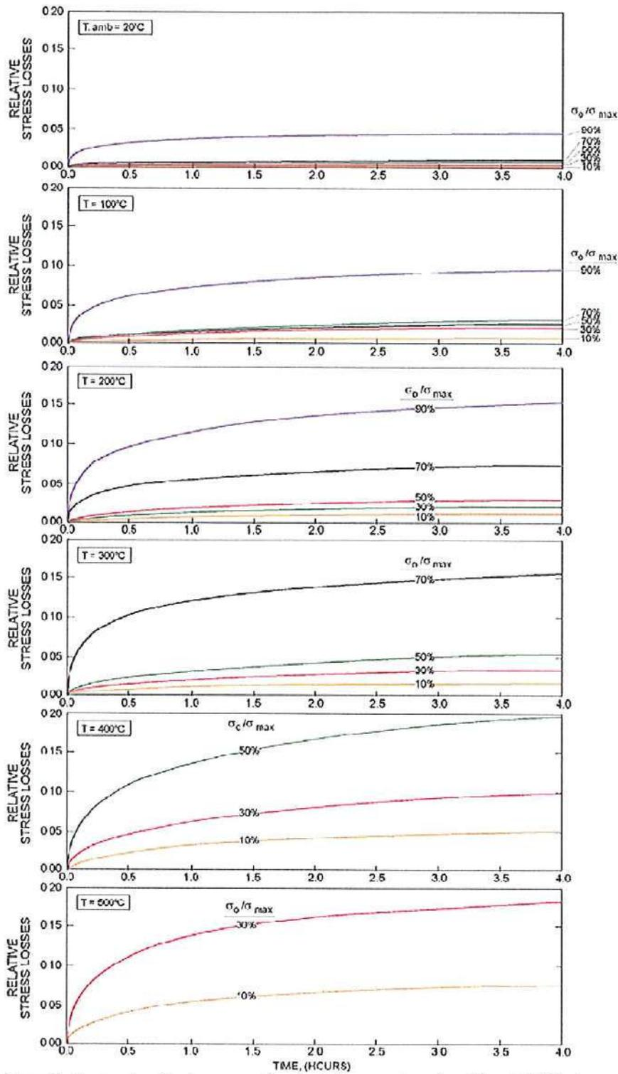
Figure 2. Stress-relaxation losses as a function of temperature, for different initial stresses. The relative values are given as stress loss/strength
