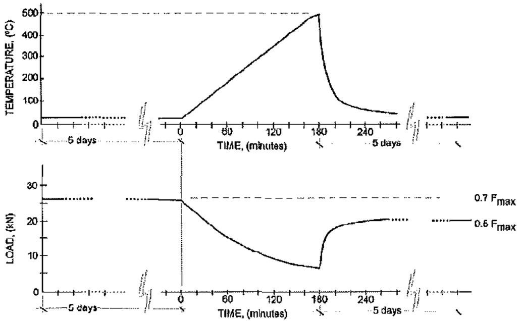
Figure 1. a) Time-temperature curve endured by the steel wire during the fire simulation. b) Evolution of prestressing load during the fire simulation.
