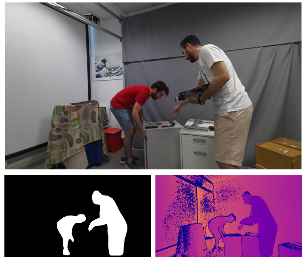
Fig. 1. A stereo dataset was generated, containing 72000 stereo pairs and the depth image associated to the left frame computed using time of flight cameras. Foreground masks were computed over them using Detectron2.
