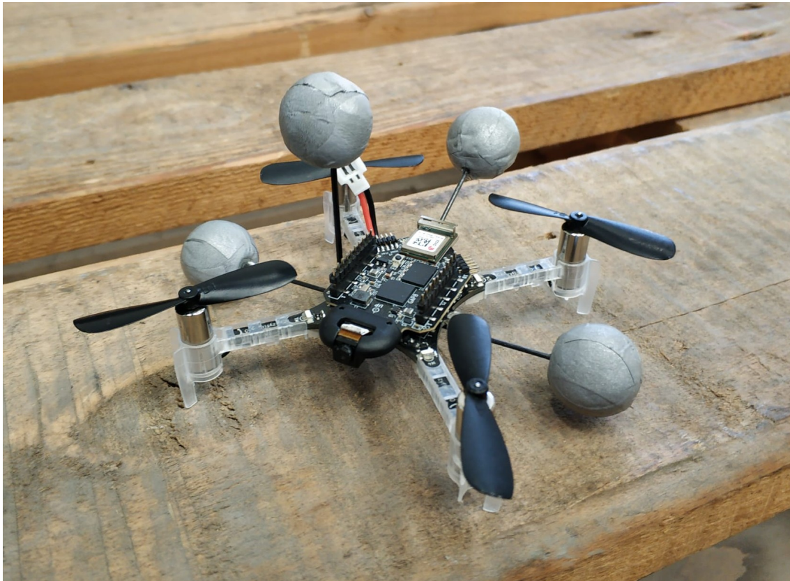
Figure 4.7 Marker geometry on the drone.
