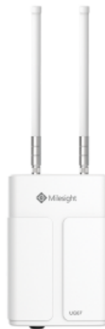
Figura 28: Milesight UG67 LoRaWan Hotspot
