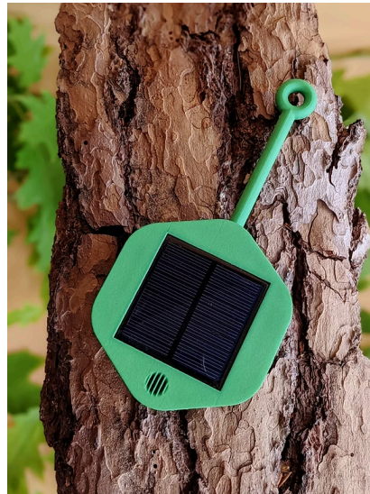
Figura 12: Silvanet Wildfire Sensor de DRYAD
