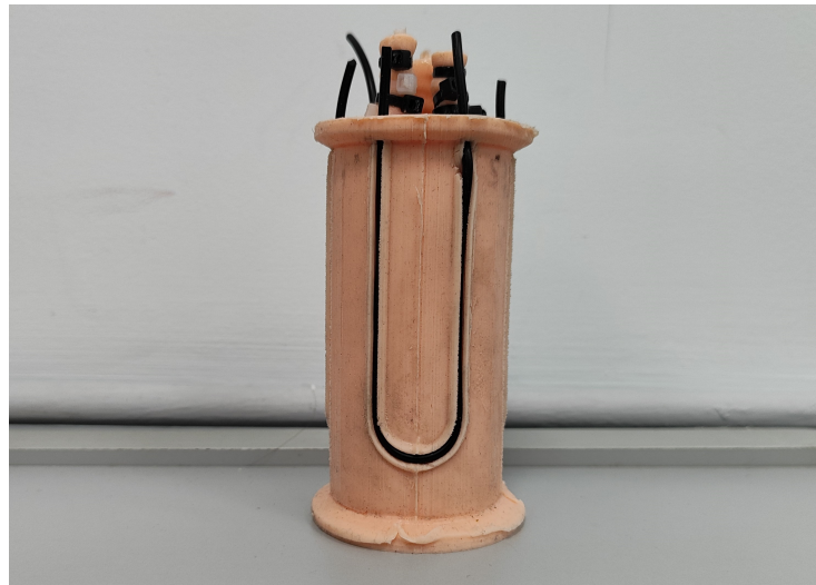
Figure 2. Conductive rubber strain sensor implemented in one of the PAUL segments. Source: Authors.
