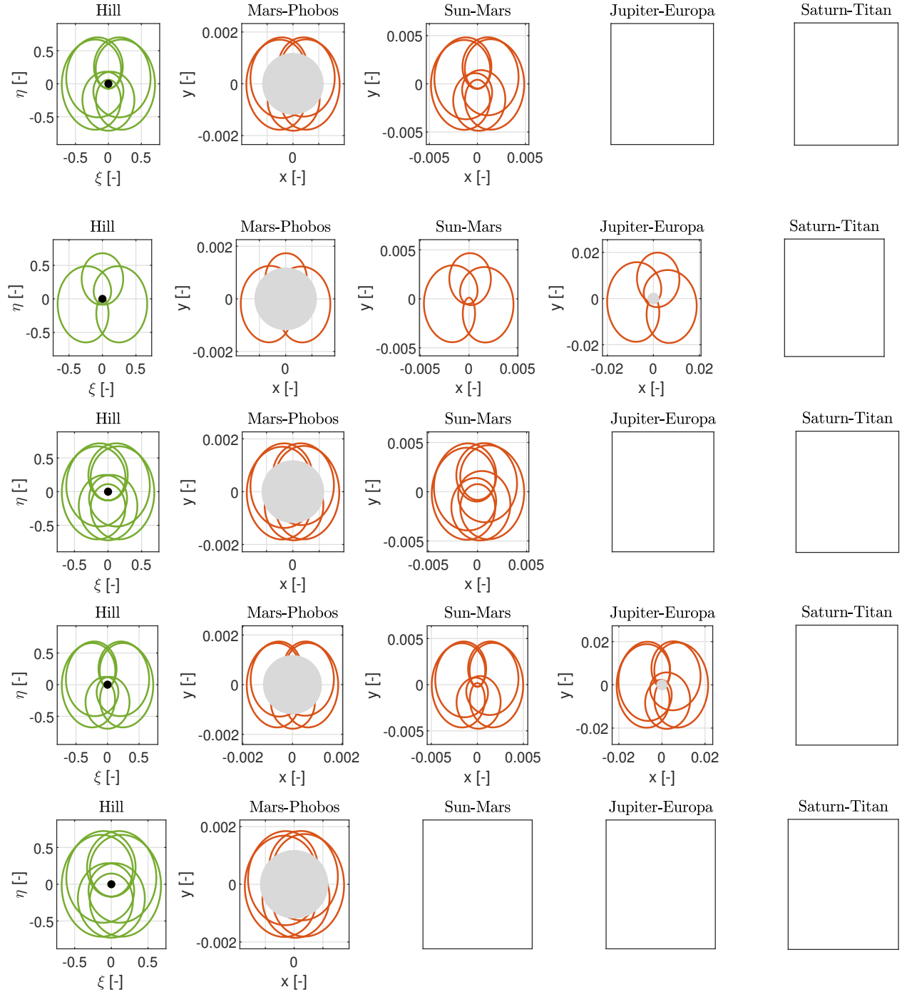
Figure D.15: WA swing QSOs in the H3BP (green), ER3BP (blue) and CR3BP (red), plotted in the \mathcal{L} frame. From top to bottom: 5:21:3, 5:24:6, 7:28:4, 8:35:5 and 9:35:5 resonances.
