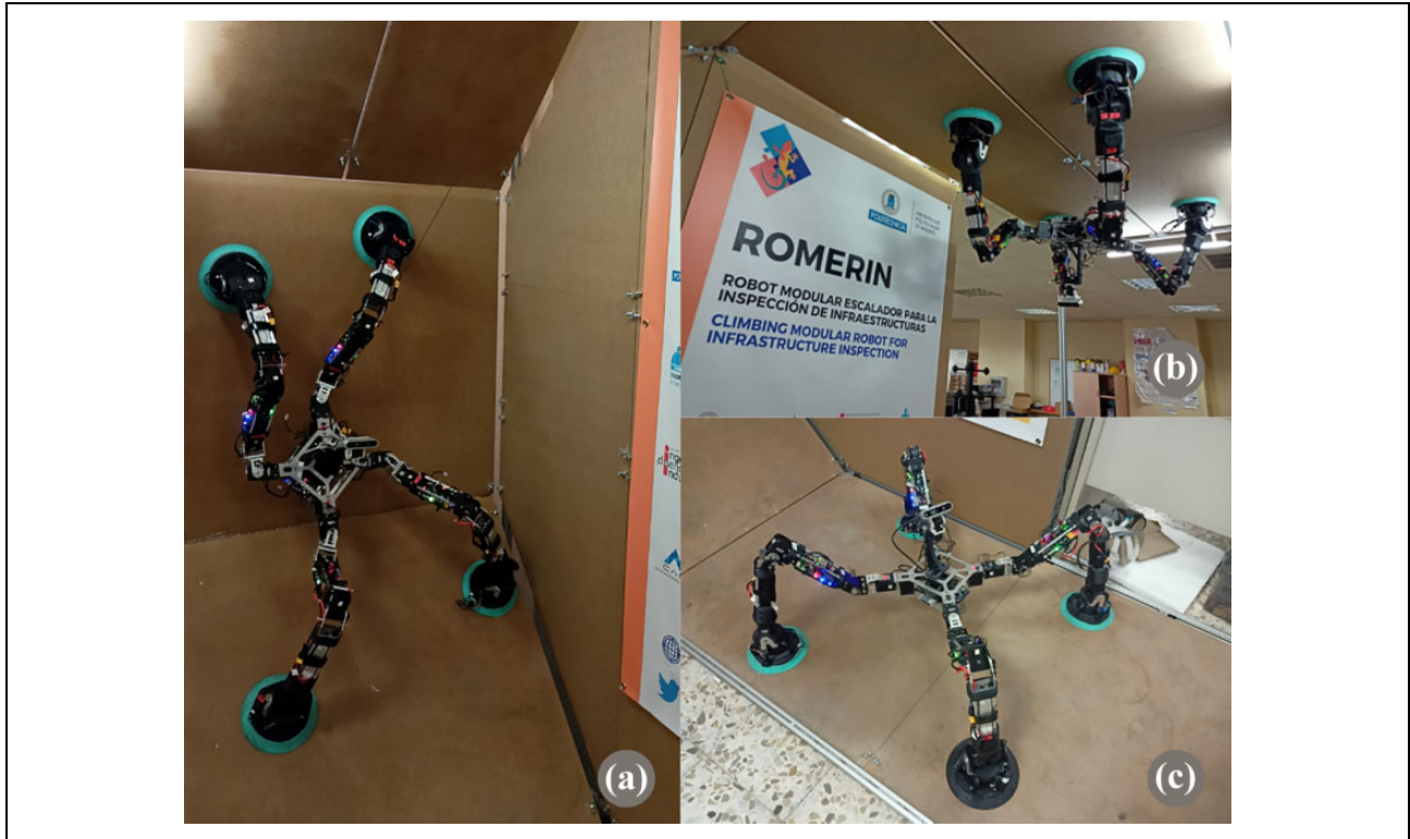
Figure 7. (a) Romerín modular robot stuck to the vertical wall of the test bench. (b) View of the robot starting up on the ground. (c) Romerín robot in an intermediate position.
