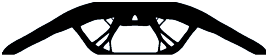
Figure 3.33: Stress-based optimization (KS, von Mises) for Figure 3.32 top left with code from [4]. Iteration 200, v_f = 0.4
