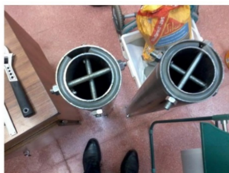
(a) Tubes prepared to proceed pouring the material that will form the core of the hybrid element.
