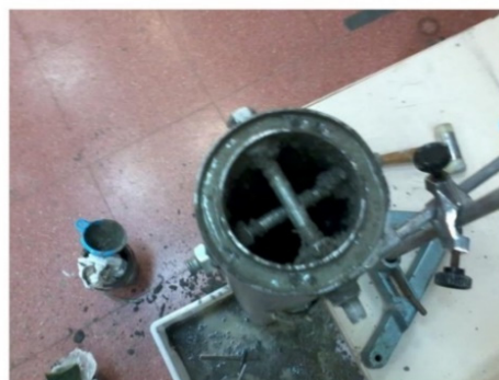
(c) Core material placed between both tubes and vibrated for its correct consolidation.
