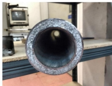
(d) Finished hybrid element, after hardening of the core and cut to the test length.
