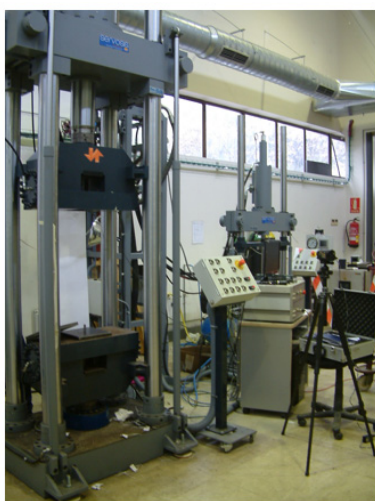
(a) Compression testing machine with load capacity of 120 t.
