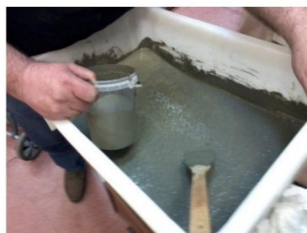
(b) Mix preparation to obtain SikaGrout-295 mortar.
