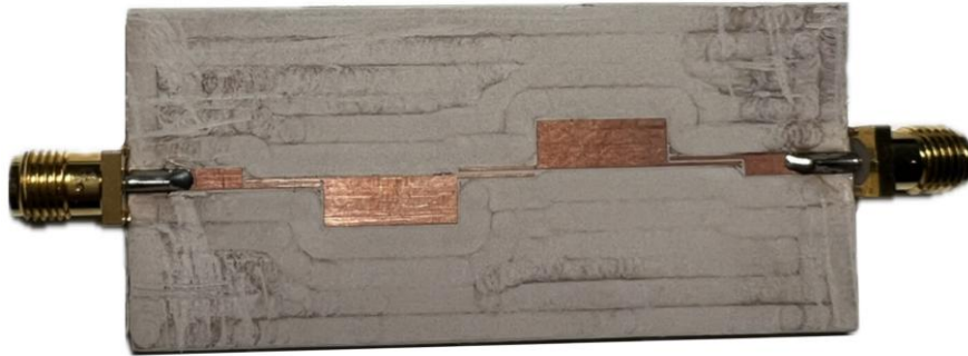
Figure 6.16. Fabricated 8th order Chebyshev UWB filter with two triple-mode SIRs.
