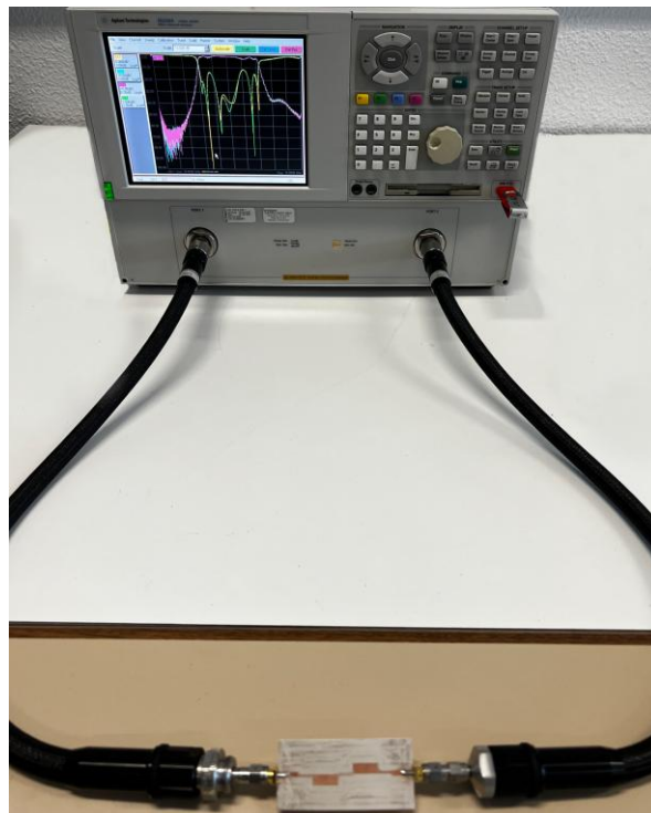
Figure 6.17. Measurement setup of 8th order Chebyshev UWB filter with two triple-mode SIRs.
