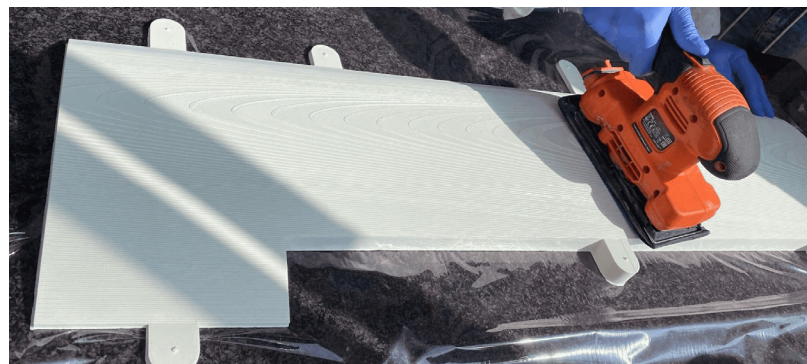
Figure 20. Sanding of the outer skin pattern surface.
