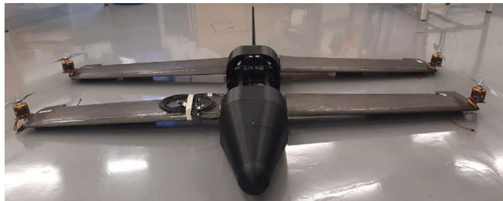
Figure 25. Final integration of the wings with the fuselage.
