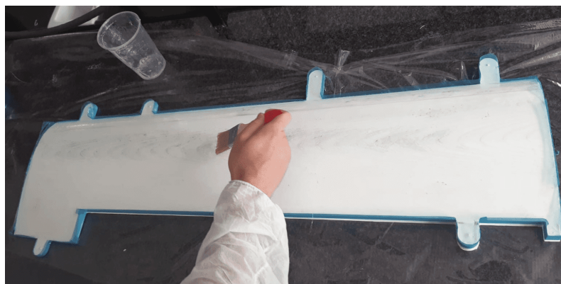
Figure 21. Application of XCR resin on the outer skin pattern surface.
