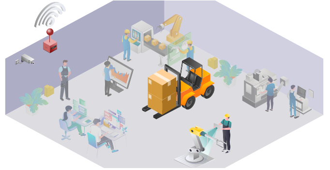
Fig. 1. Exemplary IIoT scenario with people and robots collaborating. The Wi-Fi Access Point provides connectivity to the time-sensitive flows of the camera, forklift and robotic arms (highlighted icons).
