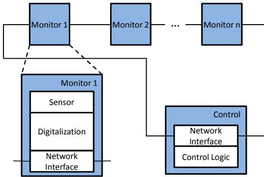
Fig. 2. Network architecture for the boundary-scan style.
