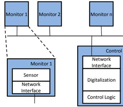
Fig. 4. Network architecture for the digitalization resource sharing.
