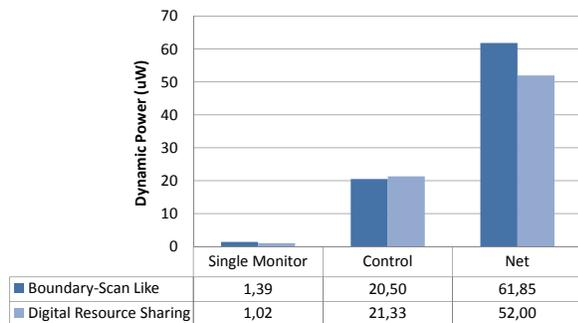
Fig. 8. Power results and comparison.
