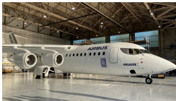
Figure 1.10: E-Fan X, a conceptual example of Hybrid Electric Aircraft (HEA), particularly of parallel partial hybrid (Image source: ©Airbus Group [44])
