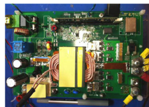
(c) DAB. 360-420 V, 98 % efficiency, 2 kW. FREEDM Systems Center, North Carolina State University [92]
