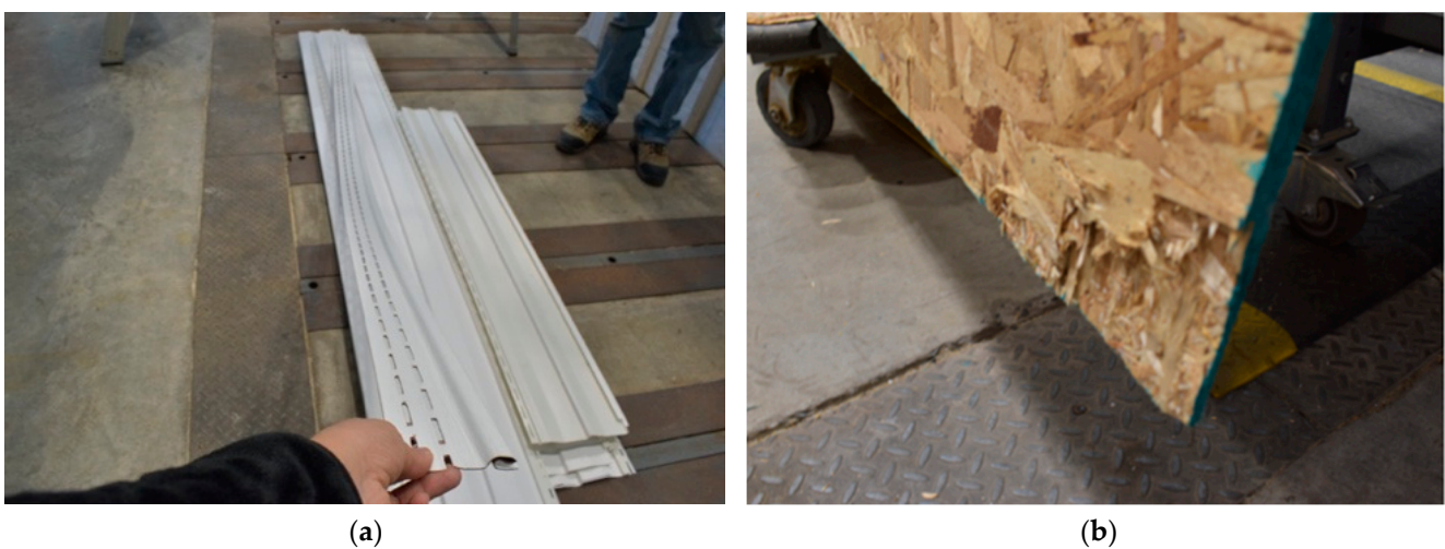
Figure 10. Material condition: (a) good condition of vinyl siding with minor edge cracks from fixings; (b) damage to the corner of the OSB board due to nails.
