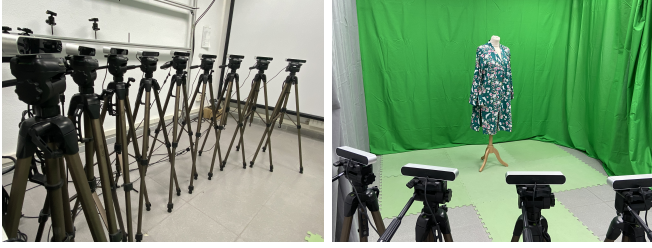
Fig. 3. FVV Live capture module setup. 9 stereo cameras (Stereolabs ZED) capture both the color and depth information from the scene in a green cyclorama setup to ease the process of real-time segmentation.
