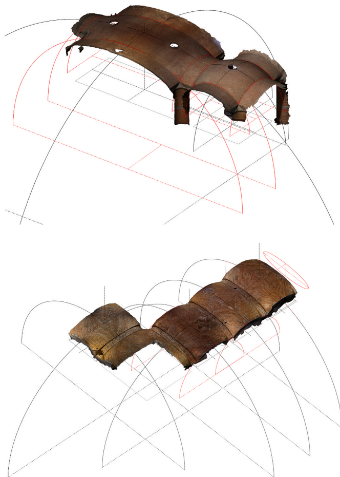
Fig. 4. Study of lines. A: Circular arcs in perimeter and axial sections of case 3 (Mole Antonelliana). B: Circular arcs in axial sections and lowered ellipses in perimeter arches of case 6.
