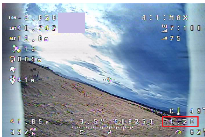
Figure 32. Measured peak acceleration of 4.2G during aggressive flight maneuvers.
