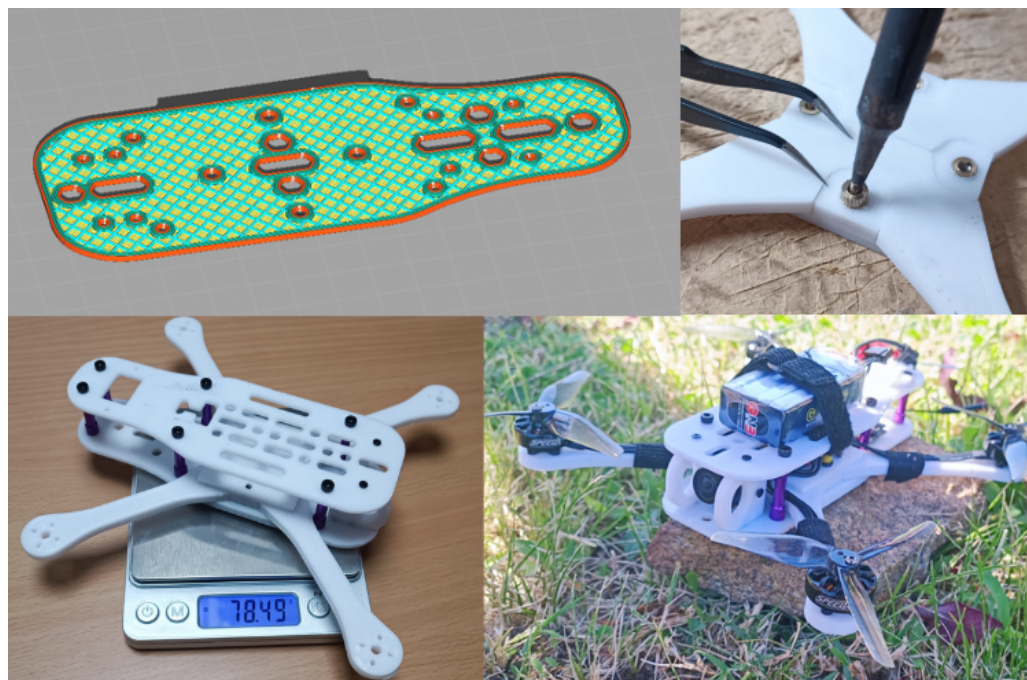
Figure 3. Steps of the fabrication process for the UAV structure.
