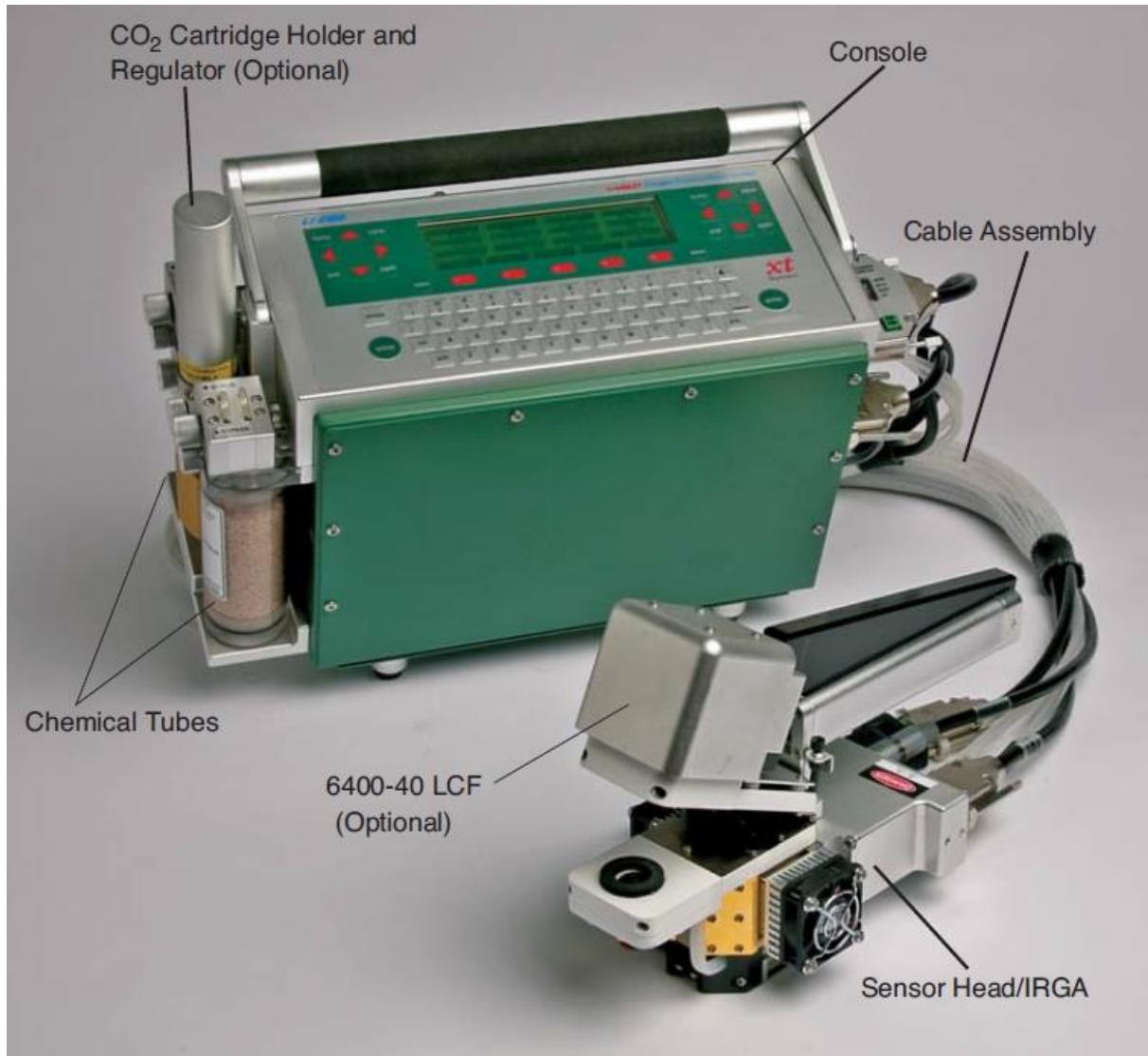
Figure 17. LI-6400XT Portable Photosynthesis System with Leaf Chamber Fluorometer (LCF). This advanced gas exchange and fluorescence system is designed to quantify photosynthetic responses under controlled conditions. The labeled components represent the core functional architecture that defines how physiological data are acquired and interpreted. Key modules include the console with integrated digital interface (user input and data logging), cable assembly (signal and power transmission), chemical tubes (air scrubbing and conditioning), and the optional CO 2 cartridge and regulator (precise control of reference gas concentrations). The 6400-40 Leaf Chamber Fluorometer (optional) and sensor head/IRGA form the analytical core, enabling simultaneous measurement of CO 2 , H 2 O, and chlorophyll fluorescence—providing a comprehensive readout of gas exchange and photochemical efficiency.
