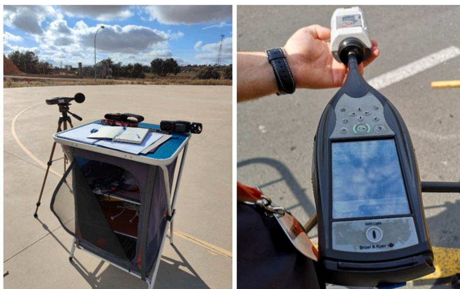
Fig. 3. Sound pressure level test setup.
