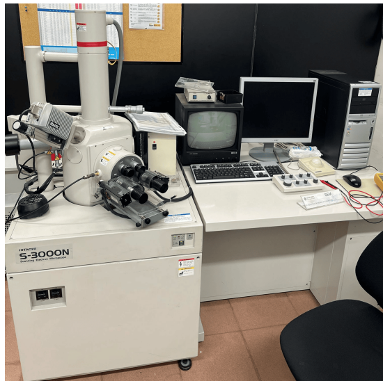
Figure 2.7: Setup of the Hitachi S-3000 N SEM.
