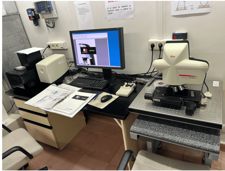
Figure 2.5: Setup of the confocal microscope Leica DCM 3D.
