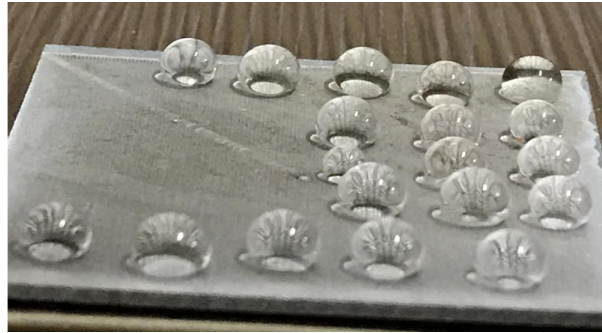
Figure 1.14: Highly hydrophobic surface obtained on an Al alloy using a nanosecond fiber laser (IPG, USA), with a pulse duration of 30 ns, scanning velocity of 3 m/s, 20 kHz repetition rate and peak fluence around 5 \text{ J/cm}^2 . Figure reproduced from ref. [100].
