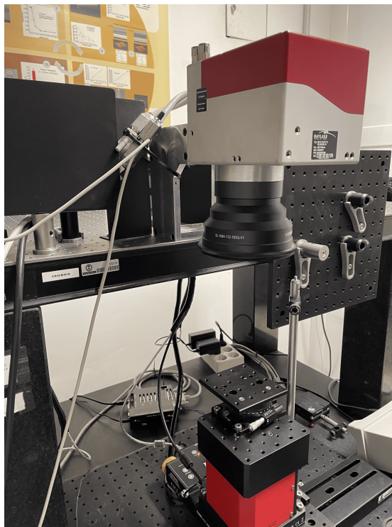
Figure 2.2: Galvanometric scanner Raylase Superscan-III, f-theta lens (Ronar-Smith, f = 163 mm) and target area. The area can also be moved in the x , y and z directions by means of a movable axis device, pictured below.
