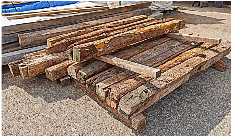
Fig. 1. Recovered European oak pieces for CLT manufacturing.
