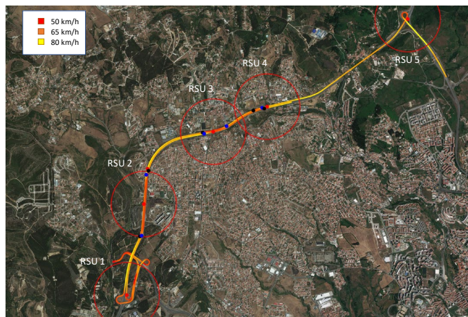
Figure 11. Route tracked by the automated and connected vehicle in the Lisbon pilot, indicating the position of the DENM messages and its range. The center of the messages matches with the position of the RSU locations.
