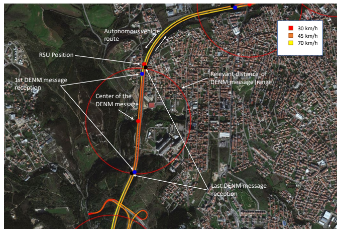
Figure 13. Detail of the automated vehicle route in the Lisbon pilot, depicting the response of the automated vehicle to a Hazardous location event in the RSU 2.
