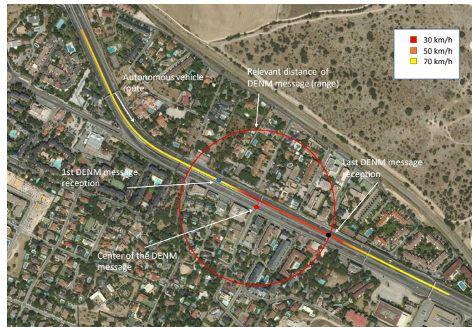
Figure 9. Route tracked by the automated and connected vehicle in the Madrid pilot, indicating the position of the DENM message and its range. The center of the messages matches with the position of the first RSU location of the corridor.
