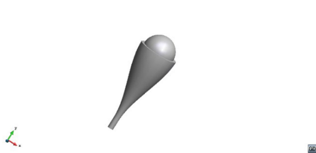
FIGURE 10 Profiled dielectric horn with a convex lens.
