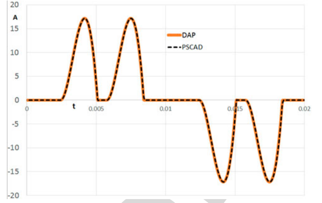
Fig. 4. Test 1: waveform for current i_a with R_d = 70 \Omega .
