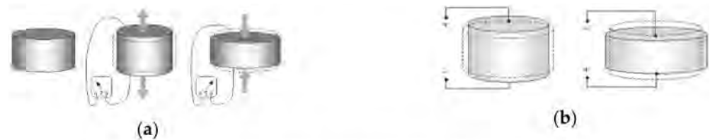
Figure 1. Piezoelectric effect: (a) Direct effect; (b) Inverse effect.
