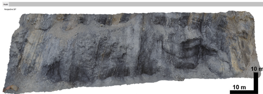
Fig. 4. Mesh and 3D model of the quarry surface from AGISOFT PhotoScan, 2014.
