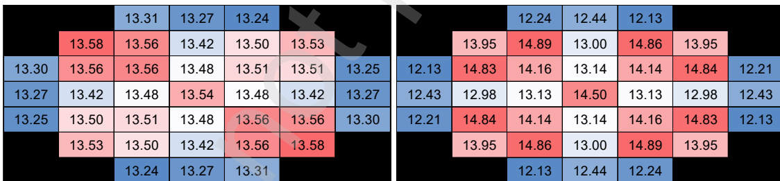
Figure 8: Radial distribution of the core mass-flow rate (TRACE-3D (left) and TRACE-3D/SCF (right))
