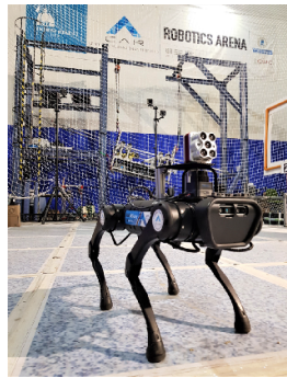
(c) Quadruped robot equipped with the multispectral camera for indoors data acquisition
