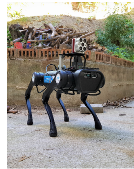
(d) Quadruped robot and the multispectral camera for outdoors data acquisition.
