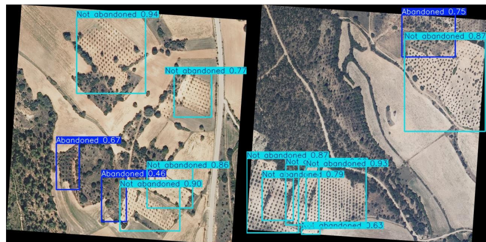
Figure 7. Results of the YOLO algorithm test. Bounding boxes indicate the detected olive groves, classified by the model as either abandoned or actively managed. The bounding boxes are overlaid on the images, each annotated with a class label and a confidence score. The results are shown without any post-processing.
